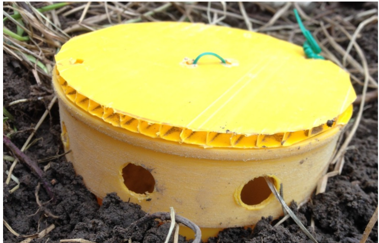
Figure B-6. Yellow bucket trap placed in the soil.
