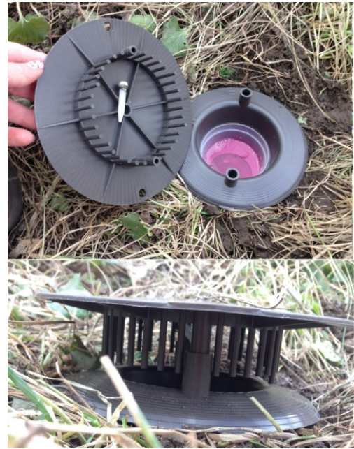
Figure B-14. Vernon pitfall trap with trap lid removed and attached.
