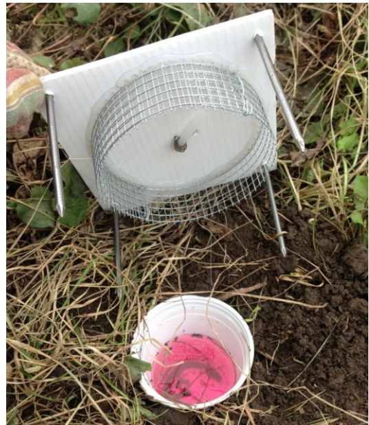
Figure B-7. Solo cup pitfall trap modified with metal mesh to exclude large bycatch.
