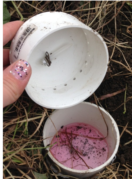
Figure B-10. PVC pitfall cup with small holes, opened to see trap inside and lure.
