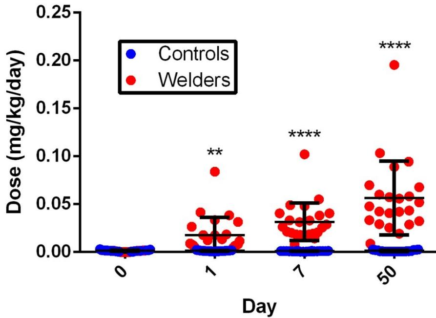
Figure 3.3 Dose (mg/kg/day) of total particle exposure in welding apprentices on sampling days 0, 1, 7, and 50 compared to controls. The dose (mg/kg/day) was calculated individually for each participant based on their weight and exposure of the corresponding sampling day. Data was collected on sampling days 0, 1, 7, and 50. Significance was calculated using a Tukey's test (\*\*  $p = 0.01$ , \*\*\*\*  $p < 0.0001$ ).
