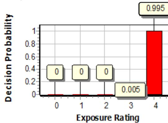
Figure 3.4 BDA of inhalable and respirable particles for welders on sampling days 1, 7, and 50 (n = 69). The following charts demonstrate that a category 4, > 5% exceedance of the OEL can be rejected with > 99% confidence for inhalable particles. When comparing respirable particles to AB's OEL, there is >99% chance that over 5% of the welding apprentices were overexposed.
