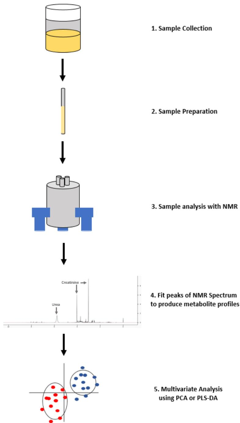
Figure 1.4 Metabolite analysis procedure with NMR. The five steps described above is the general procedure for determining metabolic profiles using NMR. Following sample collection (1), the sample is prepared and placed in an NMR tube (2) for analysis (3). FIDs undergo Fourier transform to create a NMR spectrum, which is fit for metabolite quantification (4), followed by multivariate analysis (5).
