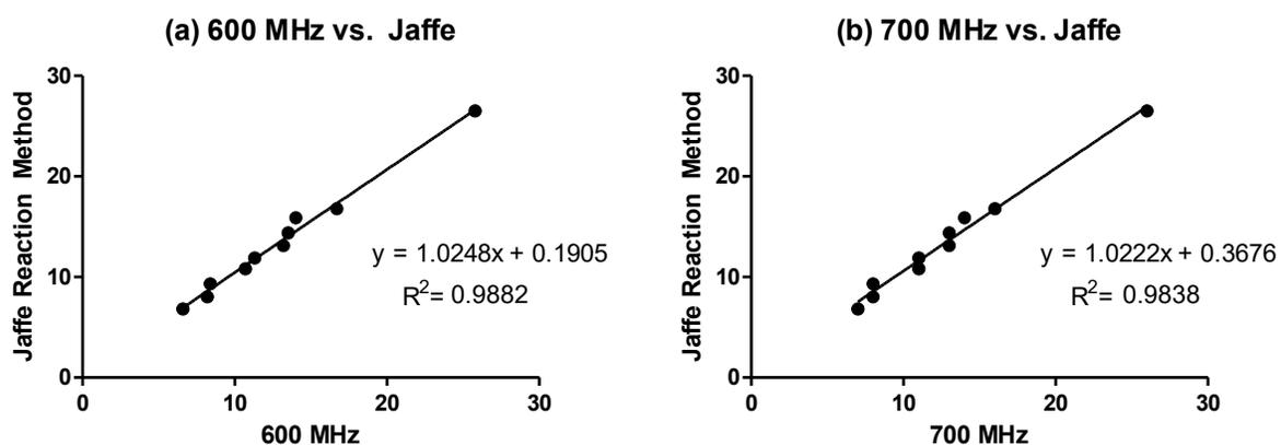
Figure 3.1 Creatinine concentration (mmol/l) comparison between Jaffe reaction method and NMR analysis (600 and 700 MHz). Urine samples were collected from 10 healthy control subjects and measured by Jaffe reaction method, 600 and 700 MHz. Creatinine values were compared using a Pearson's correlation between (a) Jaffe and 600 MHz and (b) Jaffe and 700 MHz.
