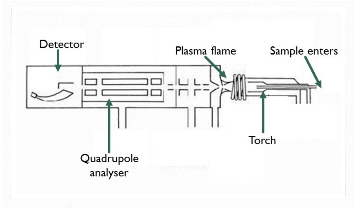
Figure 1.2 ICP-MS analysis. The sample enters on the left, where it passes through the plasma flame that ionizes the atoms, then enters the quadrupole analyzer that separates the ions based on their mass-to-charge ratio before being detected. Modified from meetcolab.com [60].
