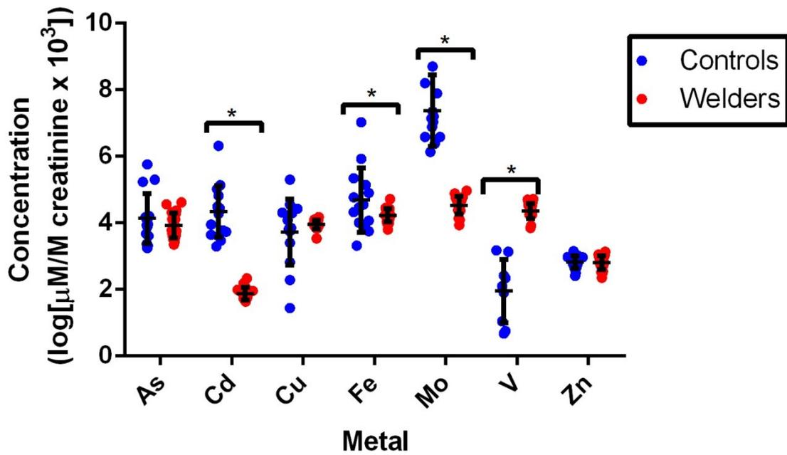
Figure 3.11 Reliable urinary metal concentrations ( $\log \mu\text{M}/\text{M creatinine} \times 10^3$ ) in controls and welders on day 50. All metals were tested using FDR ( $q = 20$ ), and Cd, Fe, and Mo were significantly ( $* p < 0.05$ ) higher in controls compared to welding apprentices, whereas V was higher in welders. All data was normalized to creatinine and log transformed.
