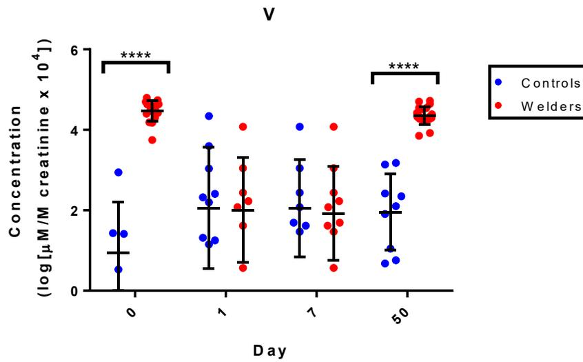
Figure 3.9 Urinary concentration ( $\log [\mu\text{M}/\text{M creatinine} \times 10^4]$ ) of V in controls and welders on sampling days 0, 1, 7, and 50. With significantly higher concentrations (\*\*\*\*  $p < 0.0001$ ) on days 0 and 50 in welders. Significance was
