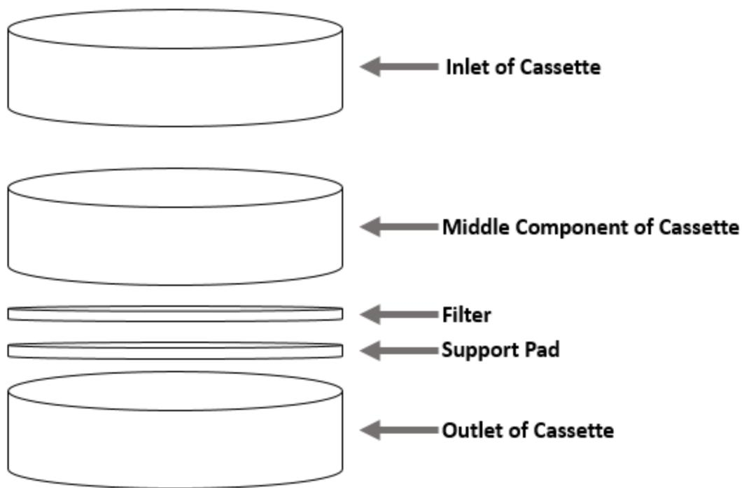
*Figure 2.1 Assembly of the three-piece styrene cassette with 37 mm support pad and filter. All components were placed together, plugs were then placed in the inlet and outlet prior to transportation to and from the sampling site.*
