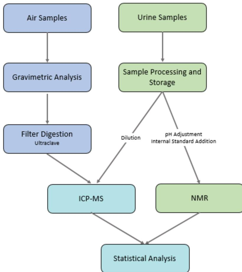
Figure 1.5 Flow chart of sample collection and analysis plan. Air sample collection and analysis is in blue, while urine collection and analysis is in green. The cyan color represents steps for air and urine sample analysis.
