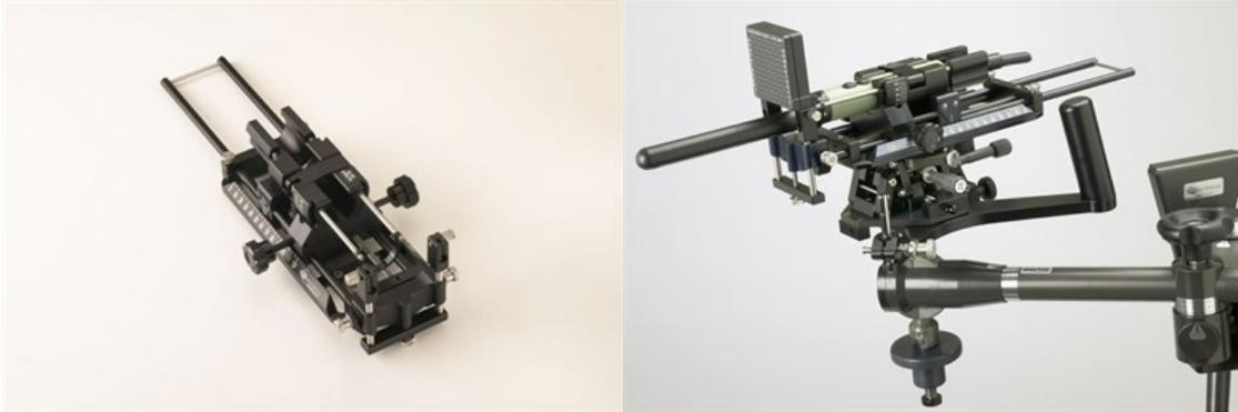
**Figure 2.4:** (left) Manual stepper for probe positioning. (right) The imaging system ultrasound transducer and support assembly: probe attached to stepper mounted on a stabilizer.<sup>6</sup> Template grid located above the probe is used only during implantation.
