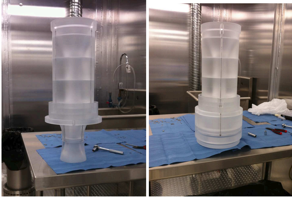
Figure 3.6: Bolted assembly of the inner (left) and outer flow guide (right) in the low-radon clean room at the University of Alberta.
