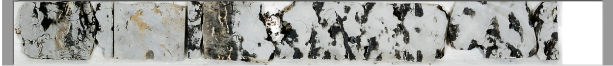
Figure 2.6: Core photo from well 4-16-85-19W4 at depth 418.05-419.00m. Core shows vugs, fracturing and bitumen staining.
