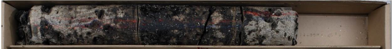
Figure 2.7: Core photo from well 7-20-85-19W4 at depth 424.25-425.00m. Core shows fracturing and vuggy porosity with bitumen staining.
