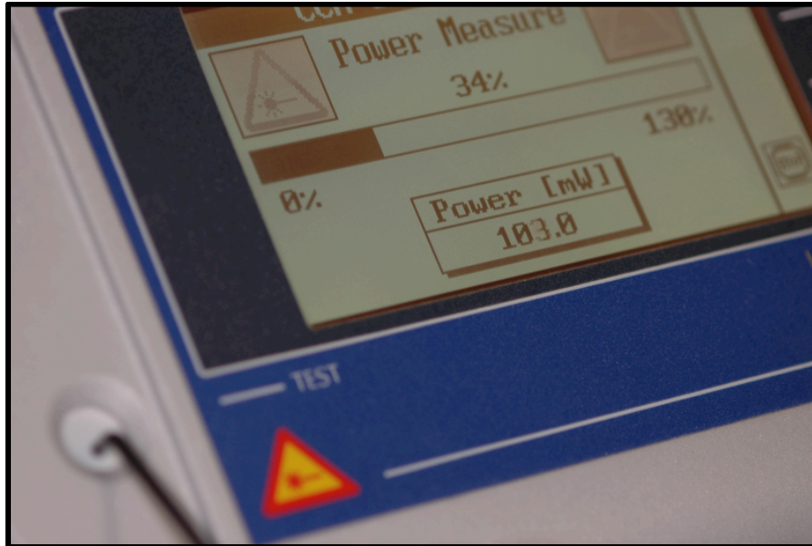
Figure 6: measuring the output power prior to each LLLT application.
