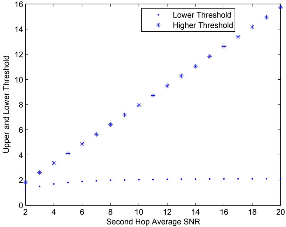
Fig. 4.2. Thresholds under different second-hop average SNR.
