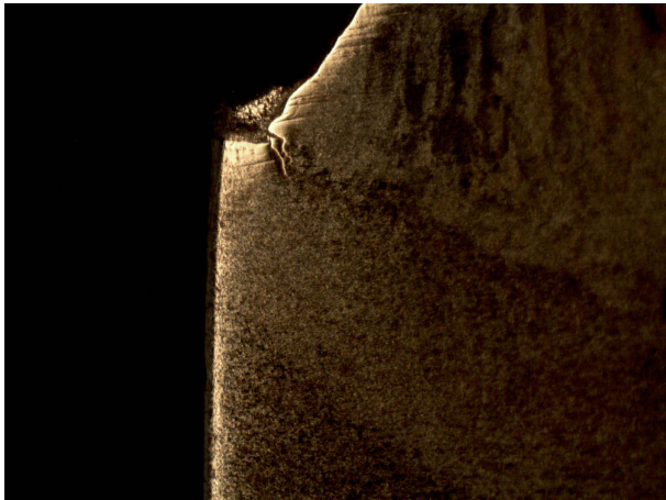
(a) Lower secondary crack
