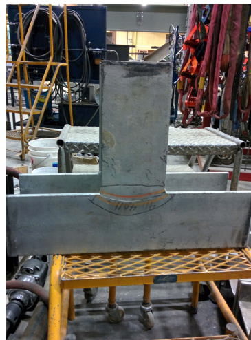
(a) Cracked Sample
