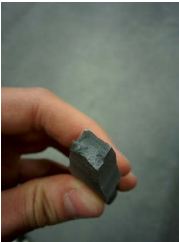
(c) Across weld, not pickled
