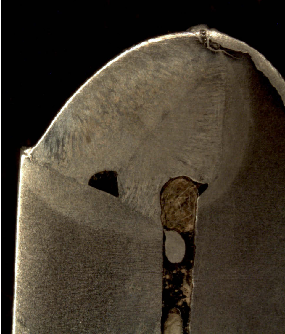
Fig. A.7: Side view of the corner joint weld
