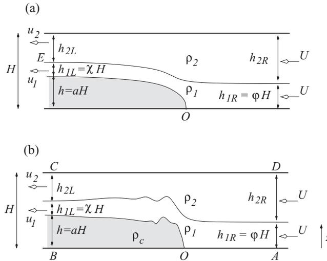
FIG. 3. Definition sketch of (a) steady two-layer flow over a semi-infinite solid obstacle; and (b) a steady, dense gravity current in a two-layer stratified ambient in which the reference frame moves at the front speed,  $U$ .
