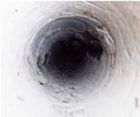
(b) Developed stress induced breakout in the direction of \sigma_3
