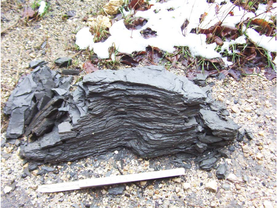
Figure D.12: Degeneration of block sample. A block of material was placed outside and carefully observed over a two week period. Maintained structure to some degree, but nearly total loss of strength.
