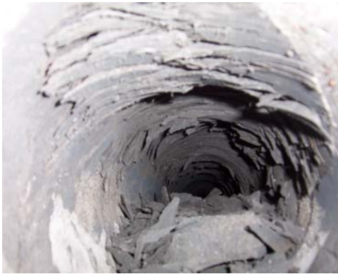
(d) Unique shape of long-term breakout for a borehole parallel to tunnel axis.
