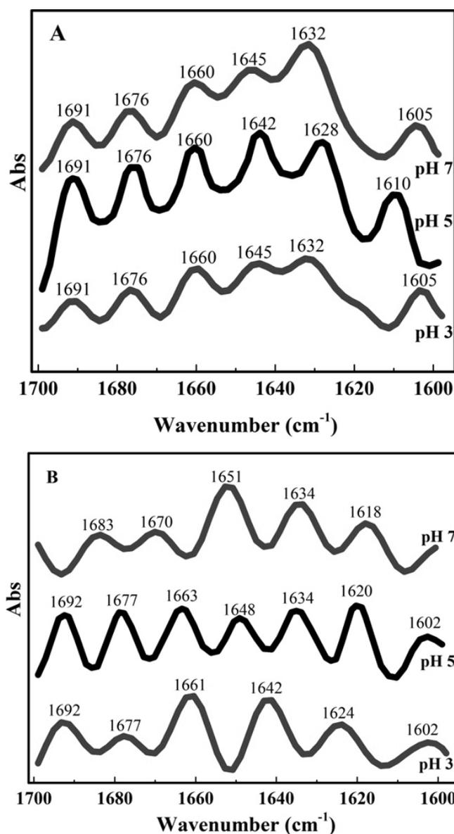
**Figure 4.6** Fourier-deconvoluted FTIR spectra of lentil legumin-like protein in solution (A) and at the foam surface (B) at pH 3.0, 5.0, and 7.0
