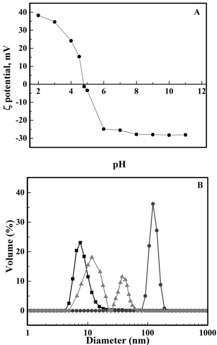
**Figure 4.2** (A)  $\zeta$ -Potential of lentil legumin-like protein as a function of pH. Values are reported as the mean of 3 samples  $\pm$  standard error of the mean. (B) Molecular size of lentil legumin-like protein in solution at pH 3.0 (square), pH 5.0 (circle), and pH 7.0 (triangle).
