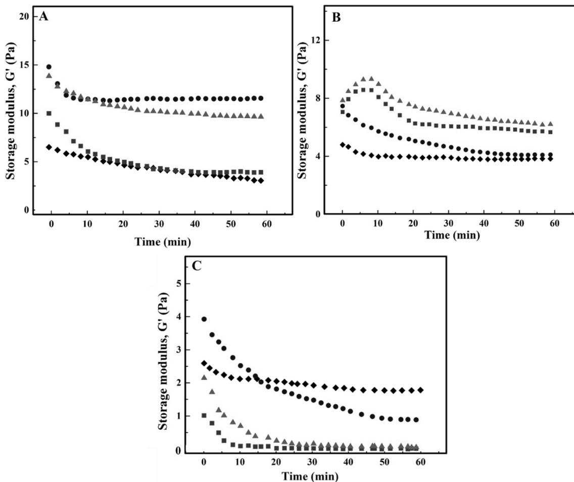
**Figure 5.4** Storage modulus of lentil legumin-like protein-polysaccharide foams as a function of time at (A) pH 3.0, (B) pH 5.0, and (C) pH 7.0 (lentil protein: diamonds, with guar gum: squares, with xanthan gum: circles, with pectin: triangles).
