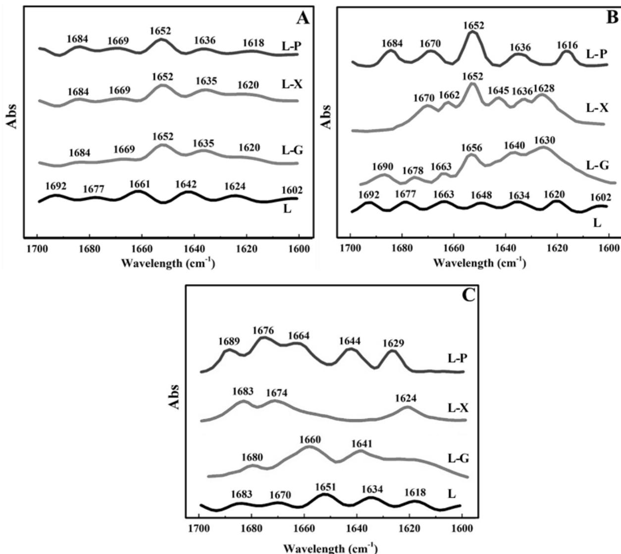
**Figure 5.6** Fourier-deconvoluted FTIR spectra of lentil legumin-like protein-polysaccharide foams at the foam surface. (A) pH 3.0, (B) pH 5.0, and (C) pH 7.0 (lentil protein: L, with guar gum: L-G, with xanthan gum: L-X, with pectin: L-P).
