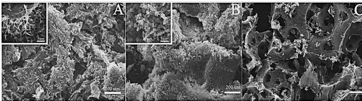
**Figure 4.7** SEM micrographs of foams produced from lentil legumin-like protein at (A) pH 3.0, (B) pH 5.0, and (C) pH 7.0.
