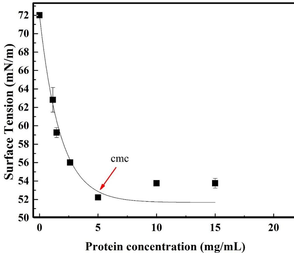
Figure A2.1 Critical micelle concentration (cmc) of lentil legumin-like protein ( $R^2$ : 0.99).
