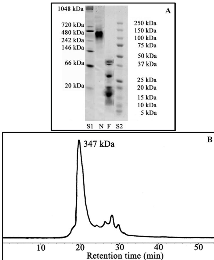
**Figure 4.1** (A) Lentil legumin-like protein under (N) native gel and (F) SDS-PAGE gel conditions. S1 and S2 are protein molecular standards in native and SDS-PAGE gel, respectively. (B) SE-HPLC chromatogram of lentil legumin-like globulin enriched fraction.
