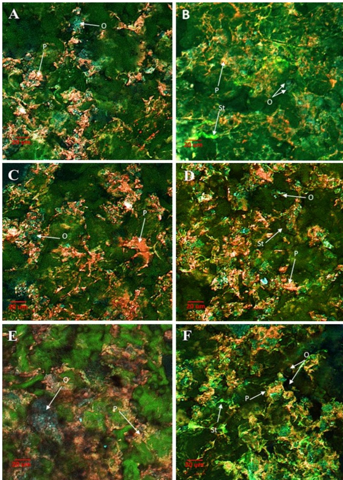
**Figure 6.6** Confocal scanning laser micrographs of muffins at day 1 (A, C, E) and 3 of storage (B, D, F). M-0-LPC (A, B), M-100-LPC (C, D), and M-100H-LPC (E, F). Triple labelled to show starch (St) (bright/dark green); protein (P) (red); lipid (O) (cyan).
