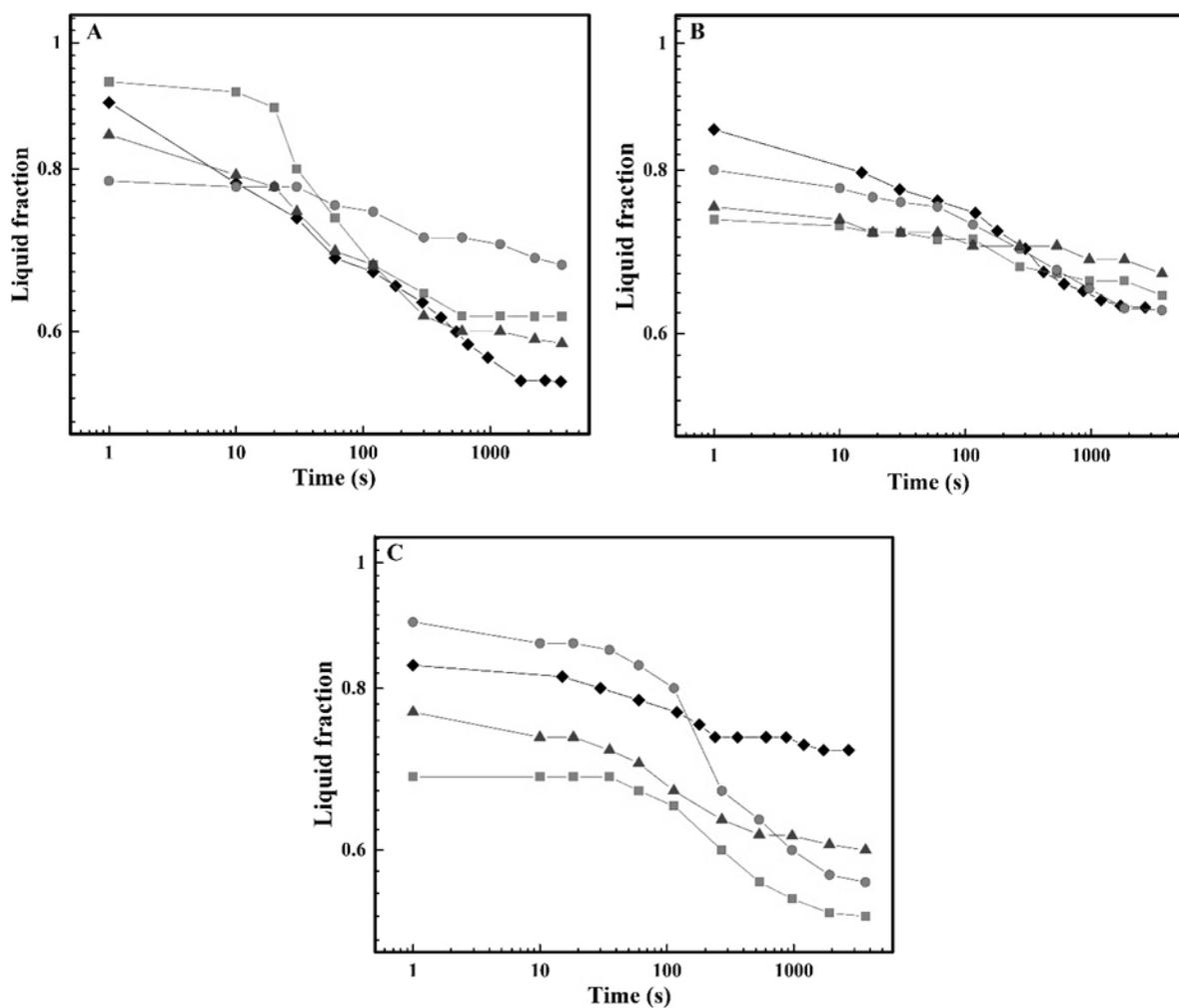
**Figure 5.5** Liquid fraction in the foams of lentil legumin-like protein-polysaccharide as a function of time at (A) pH 3.0, (B) pH 5.0, and (C) pH 7.0 (lentil protein: diamonds, with guar gum: squares, with xanthan gum: circles, with pectin: triangles).
