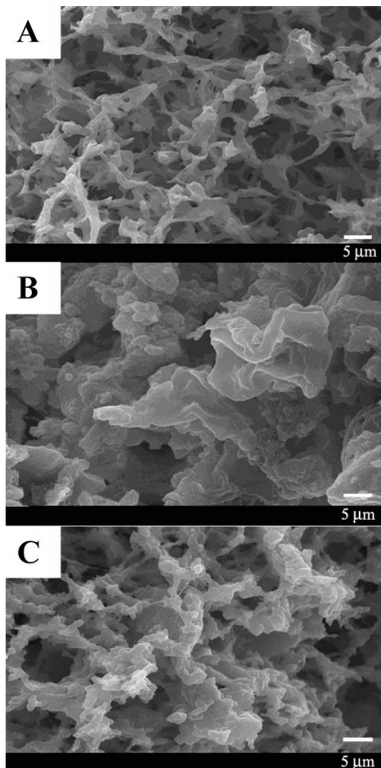
**Figure 3.5** Scanning electron micrographs of lentil protein gels prepared at pH 3.0 (A), pH 5.0 (B) and pH 7.0 (C). The protein sample was extracted at pH 9.0.
