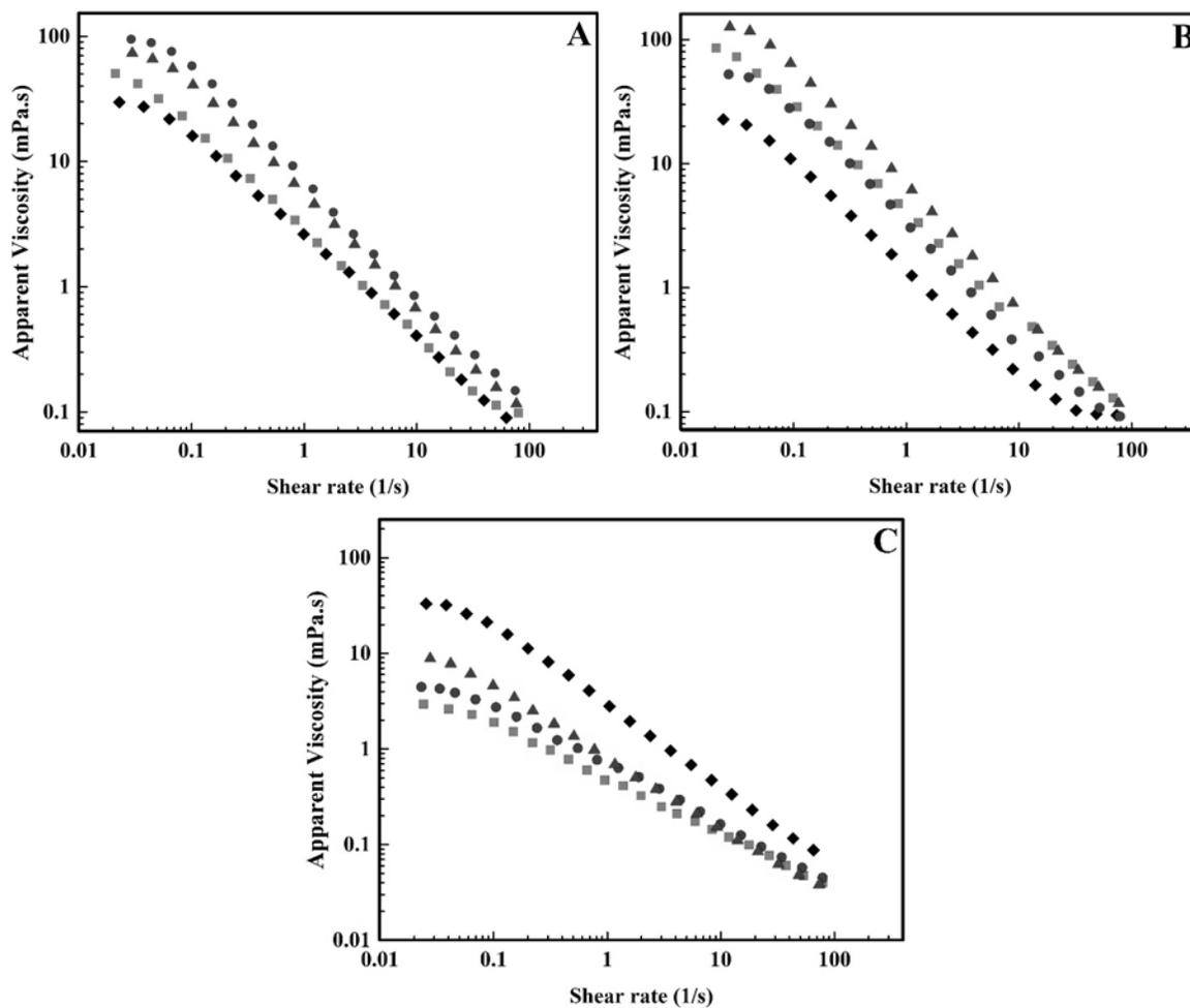
**Figure 5.3** Apparent viscosity of lentil legumin-like protein-polysaccharide foams as a function of shear rate at (A) pH 3.0, (B) pH 5.0, and (C) pH 7.0 (lentil protein: diamonds, with guar gum: squares, with xanthan gum: circles, with pectin: triangles).
