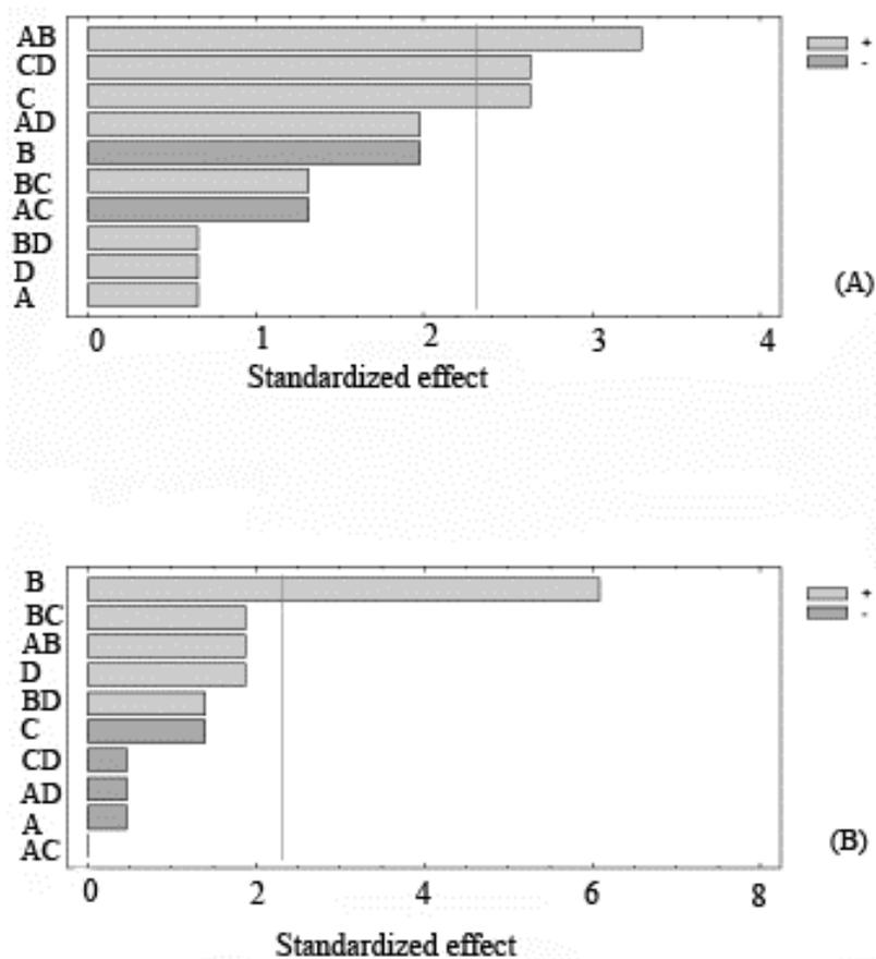
**Figure A1.1** Standardized Pareto Chart of screening design for protein content **(A)** and yield **(B)**. A: temperature; B: pH; C: solid/solvent ratio; D: time. Combinations of letters represent interactions between corresponding variables. Gray bars represent an inverse correlation between variable/response.
