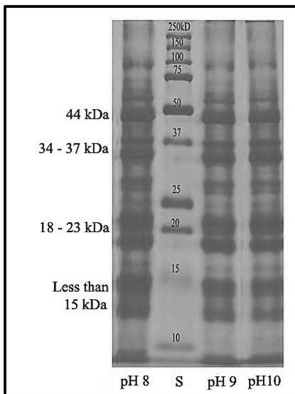
**Figure A1.2** SDS-PAGE of lentil protein concentrate under reducing conditions with 2-ME: Lane 1 (left): LP extracted at pH 8.0, lane 2: MW standard, lane 3: LP extracted at pH 9.0, and lane 4: LP extracted at pH 10.0.
