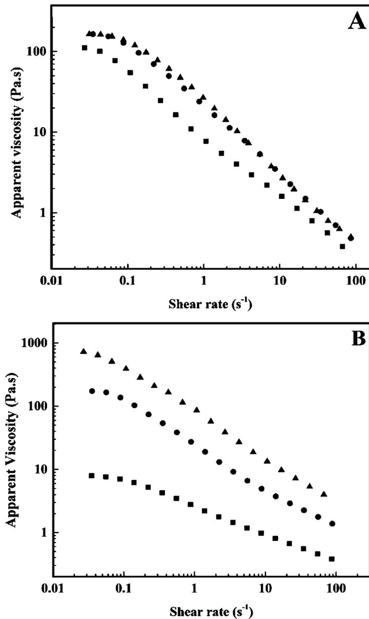
**Figure A4.1** Apparent viscosity as a function of shear rate of angel food cake (A) and muffin (B). In angel food cakes: AC-0-LPC (squares), AC-50-LPC (circles), and AC-75-LPC (triangles). In muffins: M-0-LPC (squares), M-100-LPC (circles), and M-100H-LPC (triangles).
