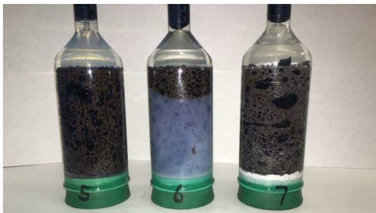
Figure 33. Nanofluids are unstable at 90°C (left: SiO_2 , middle: Al_2O_3 ; right: ZrO_2 ).
