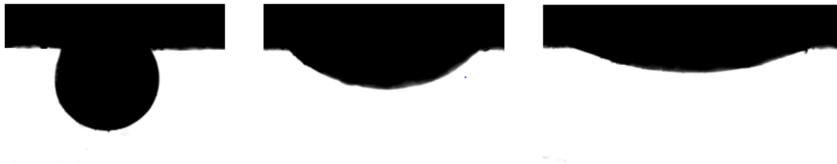
Figure 43. Oil droplets on calcite surface in C12TAB solution at 60°C, 90°C, and 120°C.
