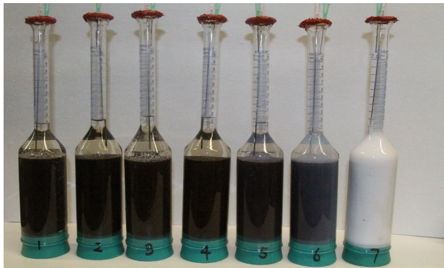
Figure 2. Indiana limestone cores in Imbibition cells (before the test).
