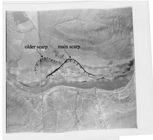
Figure 5.10: Composite image of the Red Hill slide in 1928 (centre of image), with older scarp visible to the left (south) of the main slide area. Photos courtesy of Natural Resources Canada (NRC), Roll A0291, No. 45 & 46.
