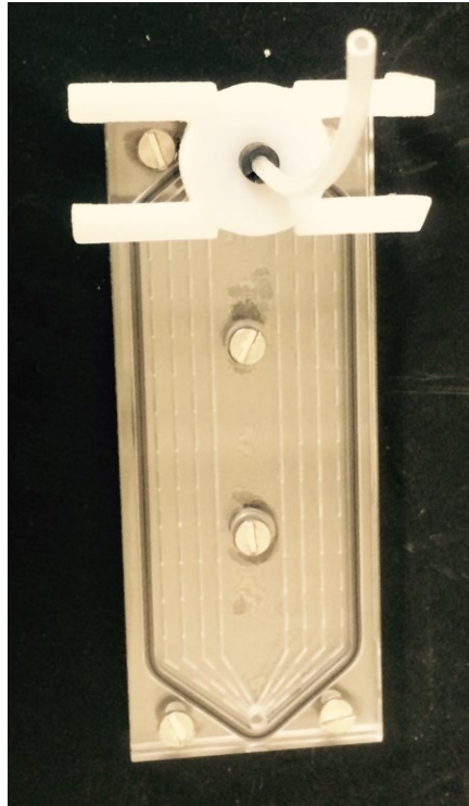
Figure 29 3D printed interconnect incorporated in one side of vapor forming microfluidic chip
