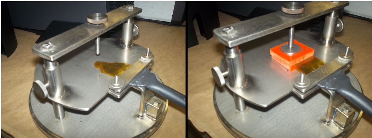
Figure 18 Thermtest sensor prior to and during testing sandwiched between test specimens fixed in test rig
