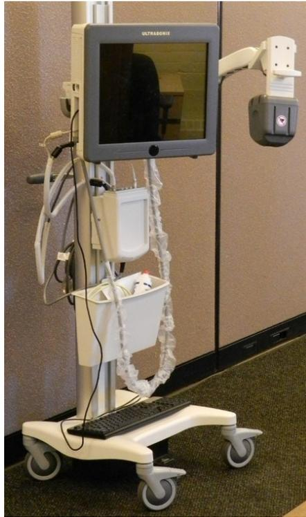
*Figure 4.1 The medical Ultrasonix SonixTablet ultrasound system.*
