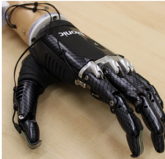
Figure 5.5 FSRs adhered to the index and thumb of the prosthetic hand
