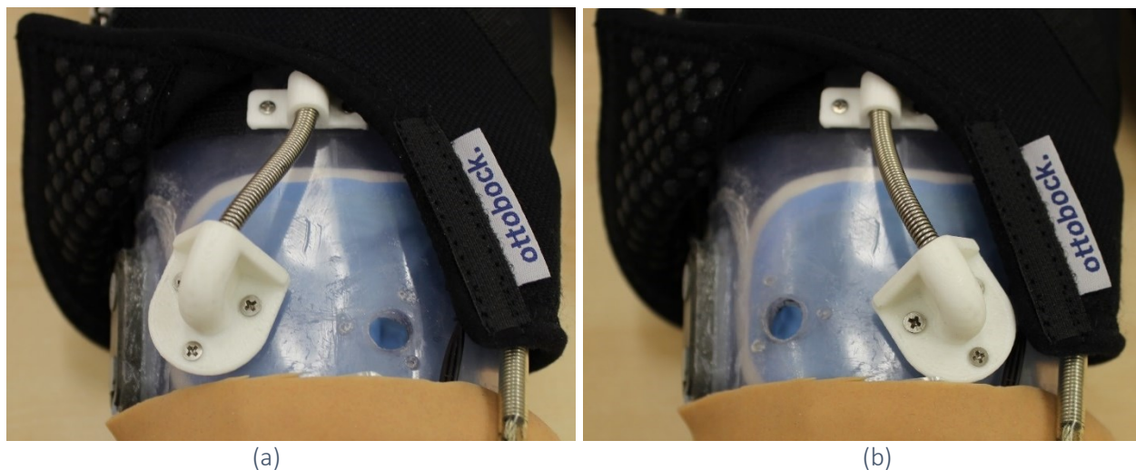
Figure 5.8 Moveable tactor head test set-up approximately (a) 2 cm from EMG electrode, and (b) 4 cm
