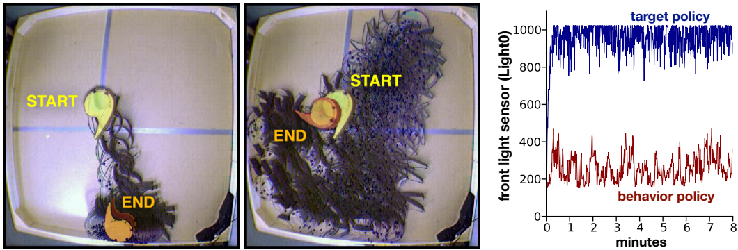
Figure 6.8: Learning light-seeking behavior from random behavior. Shown are superimposed images of robot positions: Left) In testing, the robot under control of the target policy turns and drives straight to the light source at the bottom of the image; Middle) Under control of the random behavior policy for the same amount of time, the robot instead wanders all over the pen; Right) Light sensor outputs averaged over seven such pairs of runs, showing much higher values for the learned target policy.
