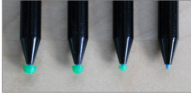
Figure 5.5. The four nibs used in the second experiment. From left to right: the 5.6 millimeter nib, the 4.4 millimeter nib, 3.5 the millimeter nib, and the 1.6 millimeter nib.
