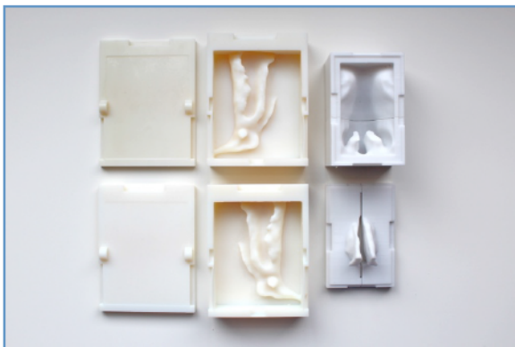
Figure 7: Prototype 2 3D printed molds for silicone casts of nose and left and right lateral wall of nasal cavity.
