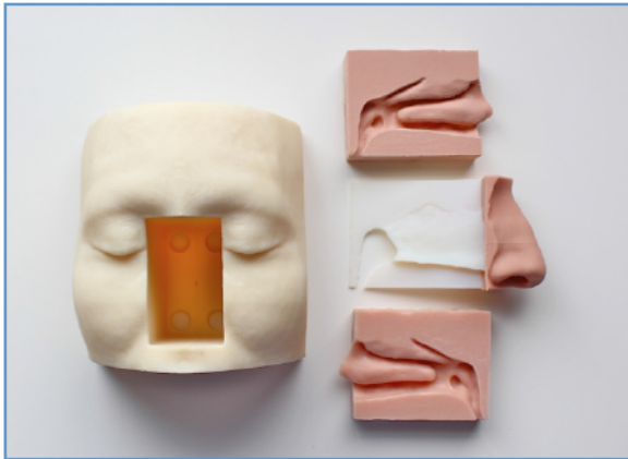
Figure 6: Prototype 2 disassembled with internal components incl. septum, nose, left and right lateral wall of nasal cavity
