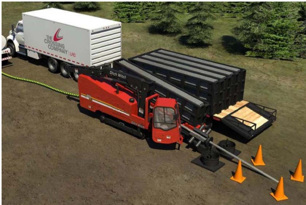
Figure 2.2. A midi-HDD with 356 kN (80,000 lb) thrust (Osbak, 2011)
