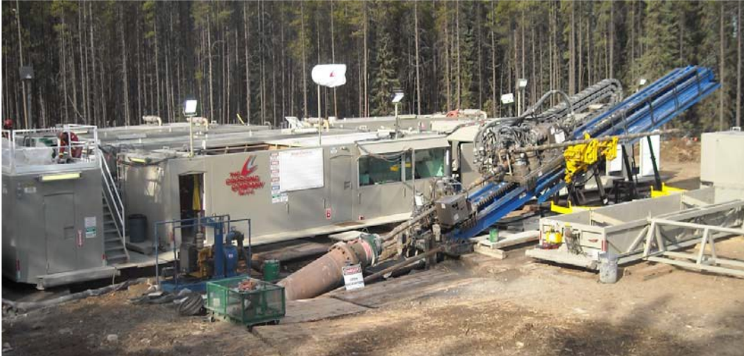
Figure 2.1. A maxi-HDD with 2780 kN (625,000 lb) thrust (Osbak, 2011)
