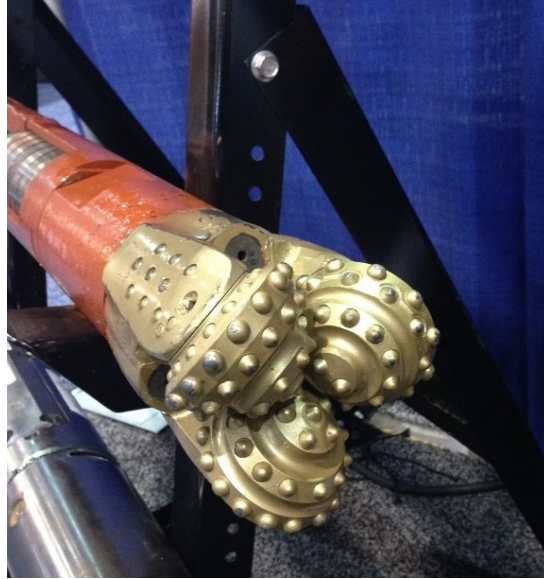
Figure 2.4. A tri-cone roller bit (Courtesy of Ditch Wich)
