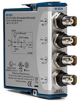
Figure 5.10. NI 9234 Module (Picture adopted from NI website)
