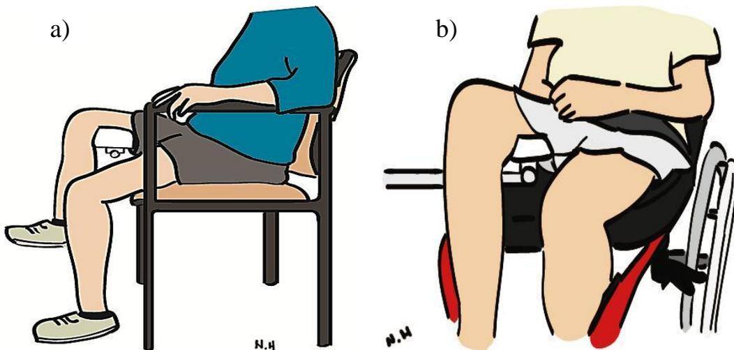
**Figure 2** Position of right leg on top of the force plate in neurologically intact subjects (a) and subjects with spinal cord injury (b). The unidirectional force transducer registered force in the downward direction.
