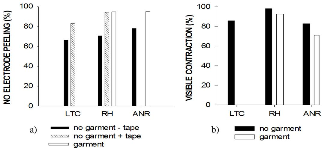
**Figure 4** Performance of IES system. Bars show overall percentages. a) Percent of no electrode edge peeling or rolling after 12 hours of being worn by the participant. b) Presence of visible gluteal muscle contractions after 12 hours of IES.
