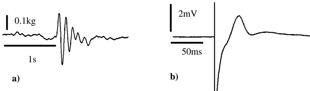
**Figure 6** Representative twitch tension (a) and corresponding M-wave (b) signals evoked by a single pulse at 100mA and 200 $\mu$ s in a person with spinal cord injury.
