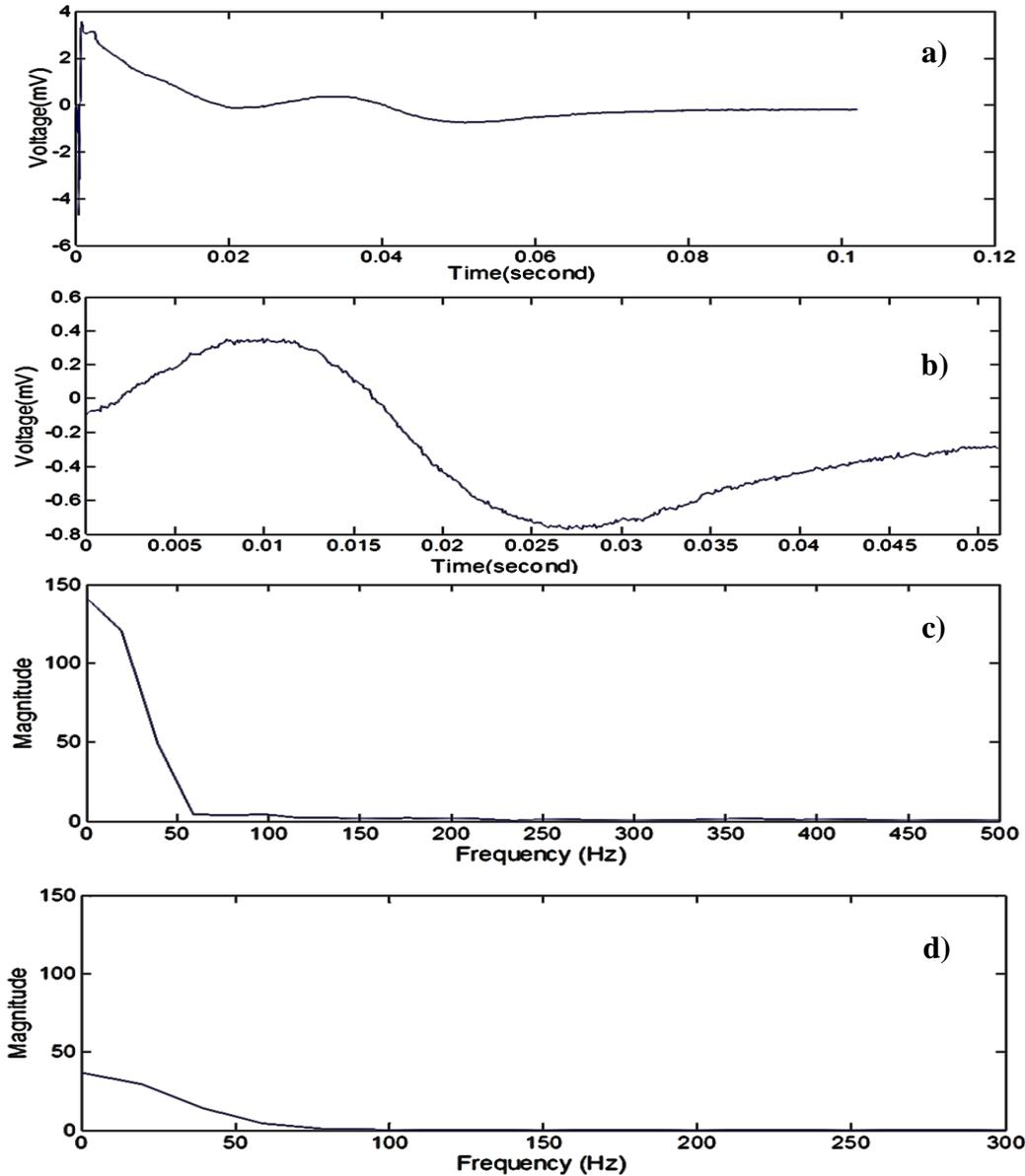
**Figure 4** The process of power spectrum density analysis of EMG data signal from one subject with spinal cord injury: a) Raw signal after template subtraction for 1 single pulse at 100mA; b) selected 512 point epoch; c) Fast Fourier Transform of selected epoch; d) Power spectrum density of selected epoch.
