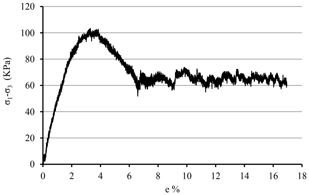
Figure B-6- Prematurely Failed test (Test F6), \sigma_3 = 34.47 kPa
