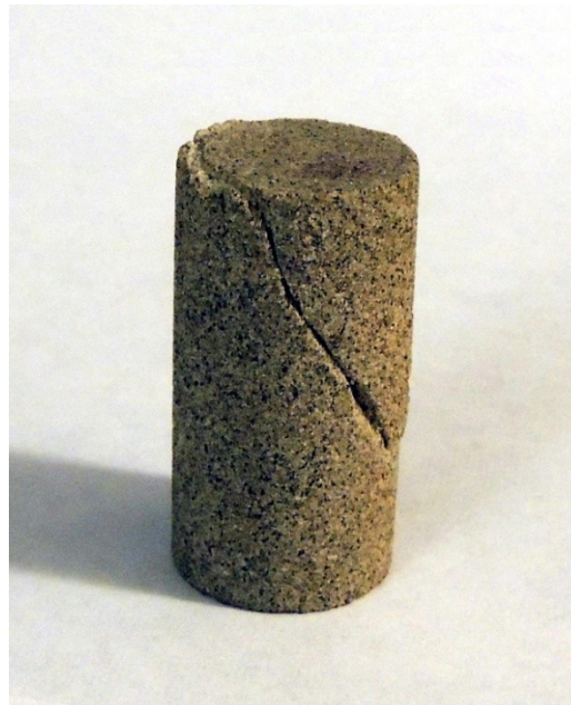
Figure 3-15- Failure mode of the intact sandstone after triaxial compression tests, D=20mm, L=40mm and \sigma_3=3.45 MPa.
