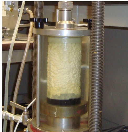
Figure 3-20- A punctured membrane with a sharp particle, without a sudden decrease at confining pressure after puncturing
