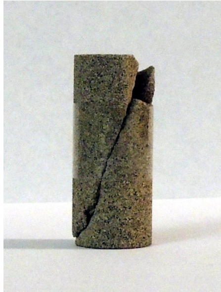
Figure 3-10- Failure mode of the intact sandstone after uniaxial compression tests, D=20\text{mm} and L=45\text{ mm}
