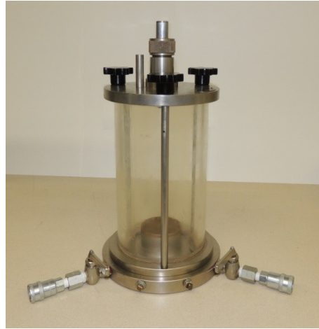
Figure 3-4- The triaxial soil cell used in this research
