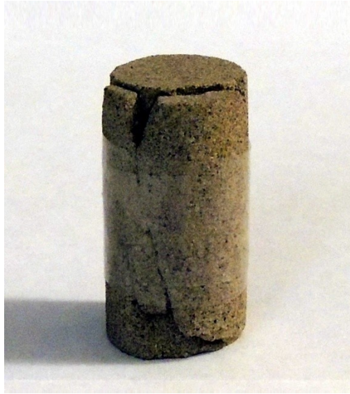
Figure 3-14- Failure mode of the intact sandstone after triaxial compression tests, D=20mm, L=40mm and \sigma_3=1 MPa.
