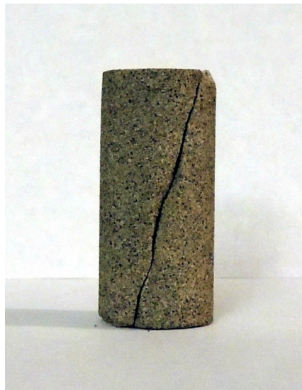
Figure 3-9- Failure mode of the intact sandstone after uniaxial compression tests, D=20\text{mm} and L=46\text{ mm}
