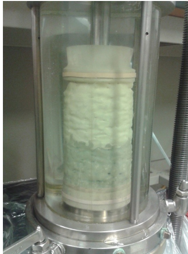
Figure 3-19- A punctured membrane with a sharp particle, with a sudden decrease at confining pressure after puncturing
