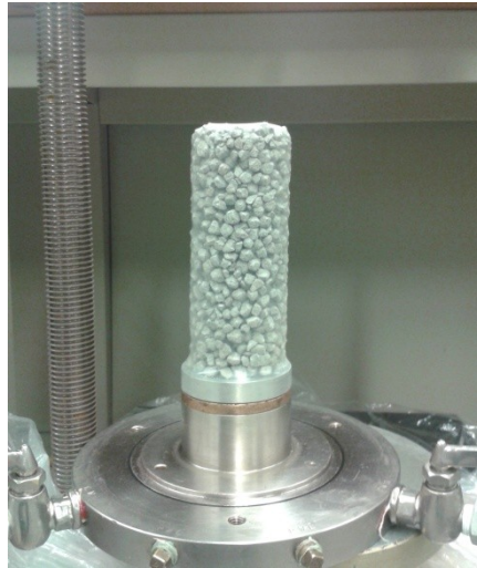
Figure 5-4- Prepared specimen for unconfined compression test on broken rock
