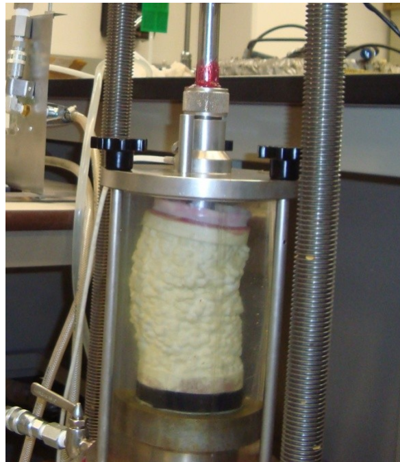
Figure 3-21- An eccentric deformation of specimen in triaxial test on broken rock
