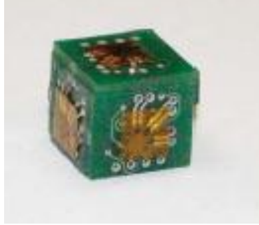
Figure 2-5 Cube measuring 10 mm x 10 mm x 10 mm for 3D strain measurement [108], Copyright © 2012 IEEE
