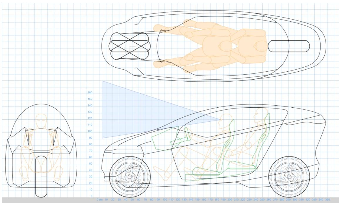
**Figure 5.9. Main component layout of RapiDES.**
